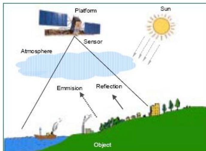
Fig. 1. Schematic representation of remote sensing technique
