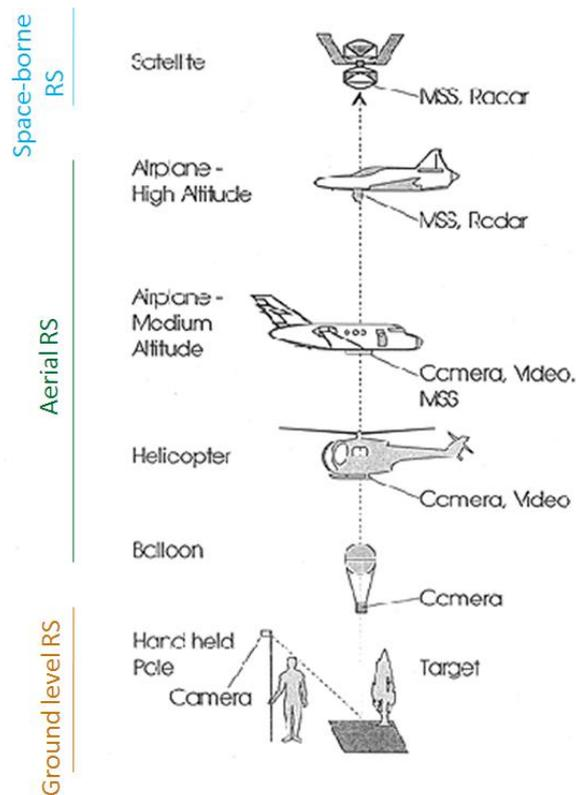
Fig. 6. Remote sensing platforms
