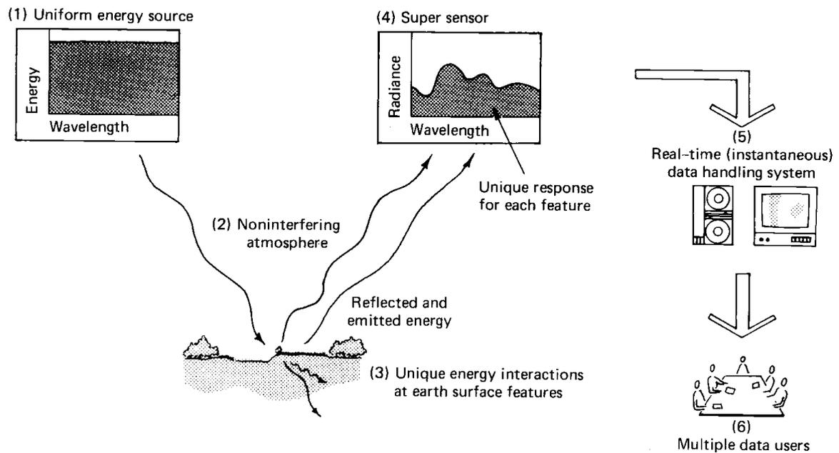
Fig. 7 Components of an ideal remote sensing system
