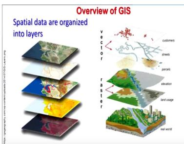
And these layers represent the different types of data which we handle in GIS platform like point data, line data, polygon data, raster data, images data and so on so forth. So, generally as we know that in GIS, spatial data is organized into layers. One important point which I want to mention; whenever I mentioned in this discussion related with this course GIS. Whenever I say data; I always mean is I am talking about the spatial data.
