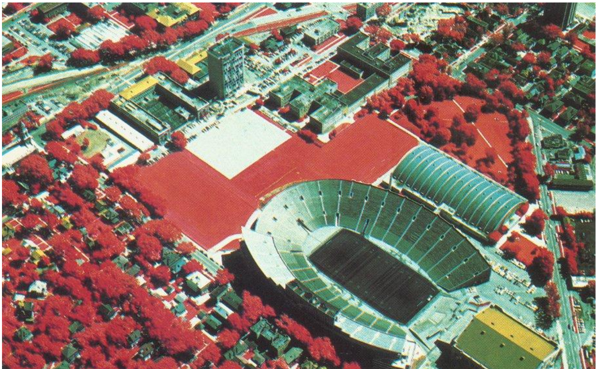
Fig. 9 Aerial photograph of a football stadium with artificial turf (a) normal colour photograph (b) colour IR photograph (from Lillesand et al., 2004)
