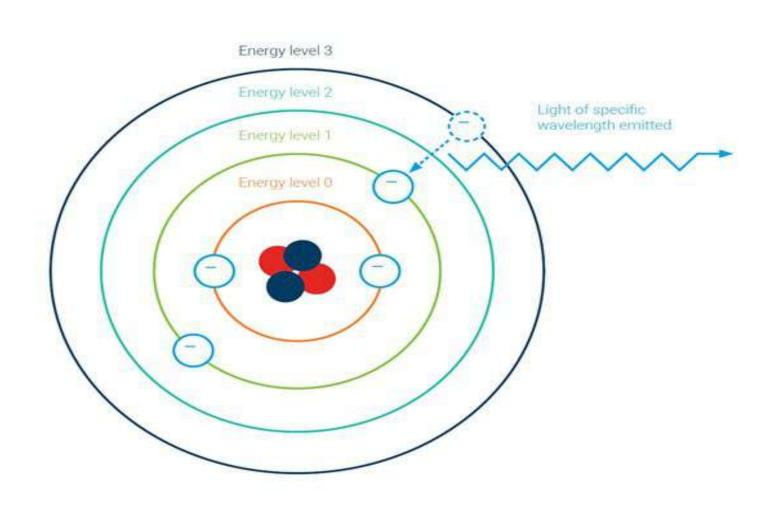
An electron is excited from the ground state to higher energy level by absorbing energy (light) at a specific wavelength. In atomic absorption spectroscopy, the wavelength of absorbed light is determined by the type of atom (which element it is) and the energy levels the electrons are moving to. How much light is absorbed is determined by the concentration of the element in the sample.
