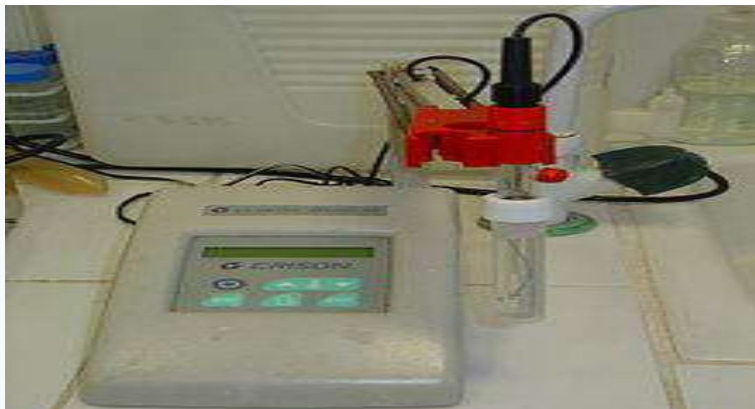
An elementary pH meter that can be used to monitor titration reactions
